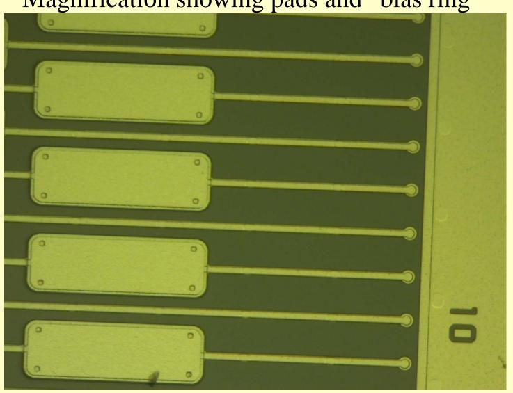
Higher Magnification showing apparent "vias" at regular intervals along length of strip
