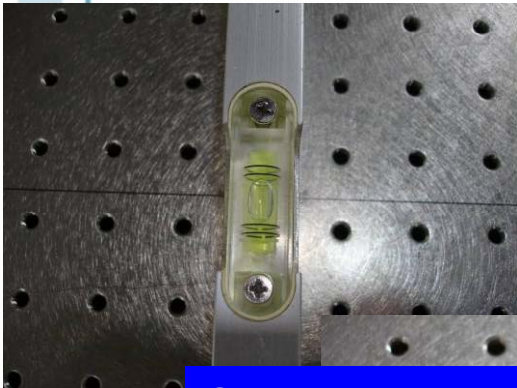
Shims ensure a levelled table
