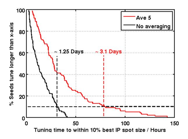
Tuning time with and without averaging of IP spot size measurements with IPBSM
