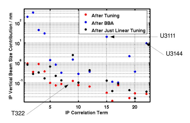
Median contributions to vertical beamsize from 100 seeds for linear + higher order correlation terms after BBA, linear knobs and all knobs.
