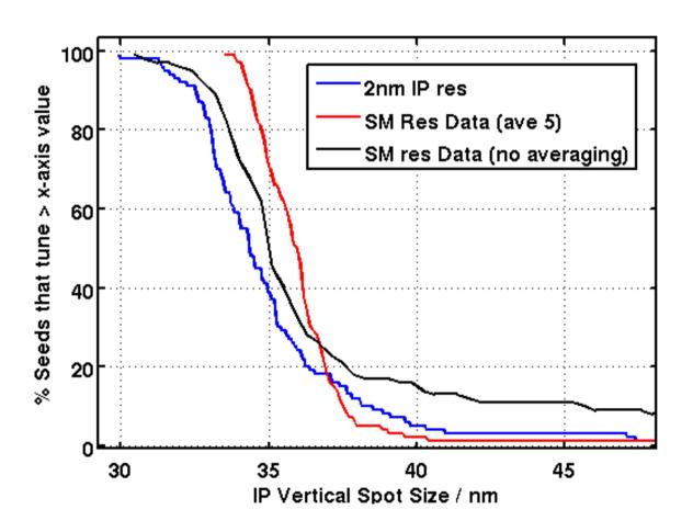
Tuning performance using IPBSM resolution data.
