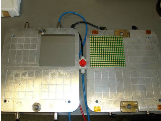
Figure 8.3- Jig, test board and wafer
