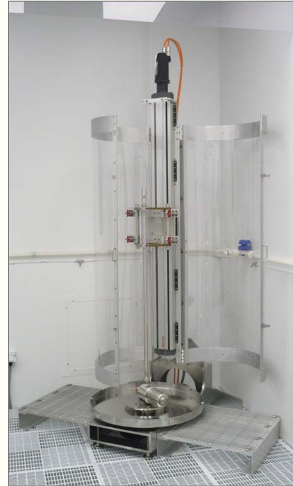
High-pressure rinsing system commissioned Oct 29
