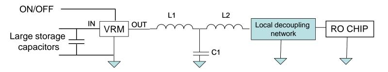
Model used to evaluate the impedance of the local power delivery network
