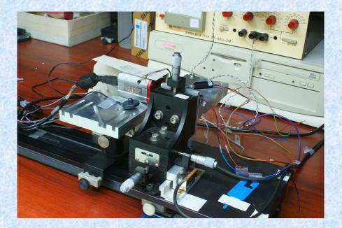
Over short distances accuracies reached: Displacements in the x-y plane: +-0.5  $\mu$ m Displacements in z direction: +- 1.5  $\mu$ m
