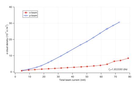
Measurements in the 17.4 m long CLEO straight with 6 wigglers. There are small differences between the propagation of the wave from center straight to its Western (dashed) and Eastern (solid) ends. The two vacuum chamber sections are not identical. Much larger differences in the low-energy electrons population are measured between circulating electron and positron beams, as expected.
