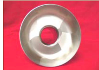
Fig. 5. Inner surface of a large grain cavity developed at JLab.
