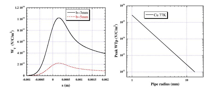
Peak of wake potential  $\sim \sigma^{1/2} b^{-3}$  $\sim 200 \text{ V/pC/m}^2$  for Cu 77K ( $\sigma$ =500 M $\Omega$ <sup>-1</sup>), radius= 2.38 mm
