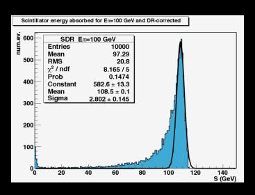
Corrected (or uncorrected) energy distribution shows major degradation of energy resolution: long tail towards low energies and a peak of punch-through pions. This is primarily caused by hadrons which interact deep inside the calorimeter, and see even smaller thickness of the detector.
