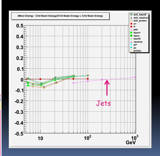
Deviations from the linearity of the response (S-B)/B for different particles as a function of their energy:
