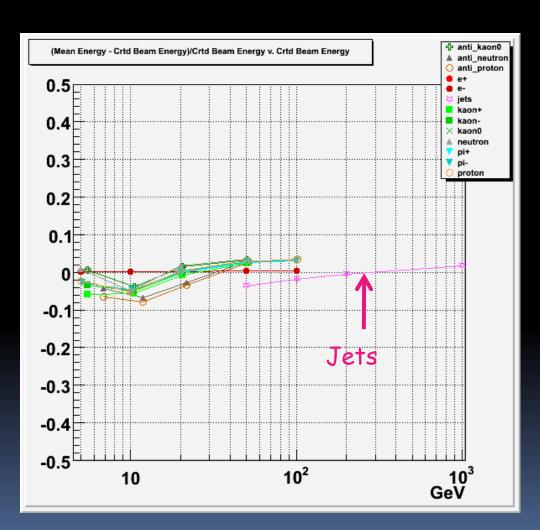
Deviations from the linearity of the response (S-B)/B for different particles as a function of their energy:
