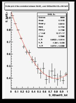
Longitudinal segmentation of a calorimeter provides information which can be used to identify and correct the leaking showers. For example (left): fraction of the observed energy of a shower correlates with the amount of the leaking energy
