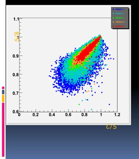
Correlation of the fraction of 'missing energy' and Cherenkov-to-scintillation ratio for showers of different energies: 10 - 200 GeV:
