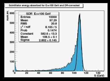
Corrected (or uncorrected) energy distribution shows major degradation of energy resolution: long tail towards low energies and a peak of punch-through pions. This is primarily caused by hadrons which interact deep inside the calorimeter, and see even smaller thickness of the detector.
