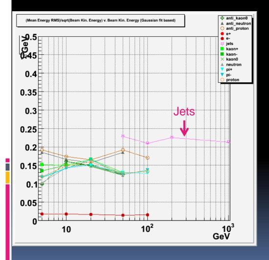
With very crude reconstruction and non-optimal global correction function: energy resolution shows no constant term and scales ∆E/E~1/ √E stochastic term in the energy resolution is ~15% for single hadrons, 2% for electrons and ~22-23% for jets there are several obvious ways to improve the energy resolution. At least in the simulated calorimeter. But can we take the simulation seriously???
