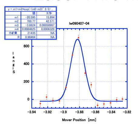
Minimum size measured=8.46um Measured Laser waist=5.96um → e beam size=~6um
