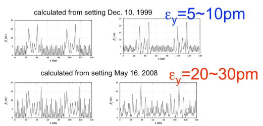
Kubo pointed out that the optics distortion is the one of the source of large emittance in DR.
