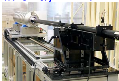
Inspection of Inner Surface
