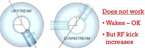
2. Compact detachable coupler unit that provides axial symmetry of the RF field and the cavity geometry in the beam channel:
