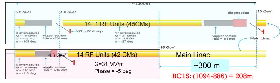
**Single-stage BC** is possible, if not support flexibility of parameter set • Changes:  $9/6 \text{ mm} \rightarrow 0.3/0.2 \text{mm}$  (RDR) to  $6 \text{mm} \rightarrow 0.3 \text{mm}$  (x20 compression)
