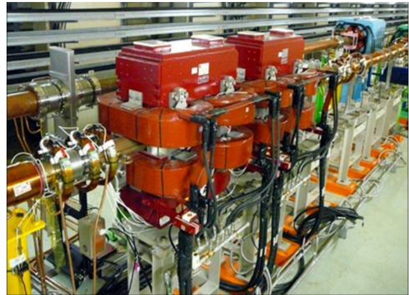
Wiggler magnets B = 0.77 \text{ T}
