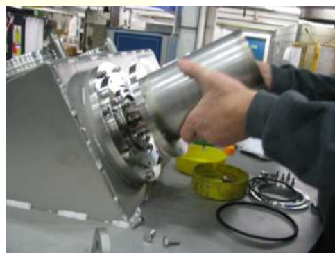
Lead head assembly and connection of power cables
