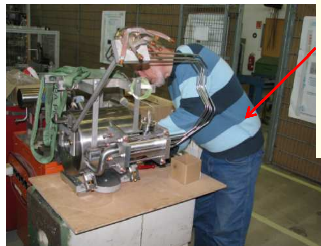
SL cables soldered to lead ends and isolated
