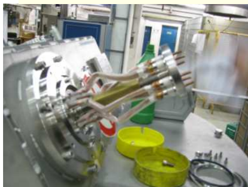
Lead head assembly and connection of power cables
