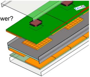
In 2007 a special slab was equipped with embedded chips (no Si wafers)
