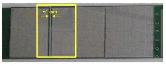
Wafers are separated by ~1 mm on both directions
