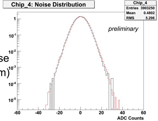
Tested global variables of noise spectra, mean and RMS
