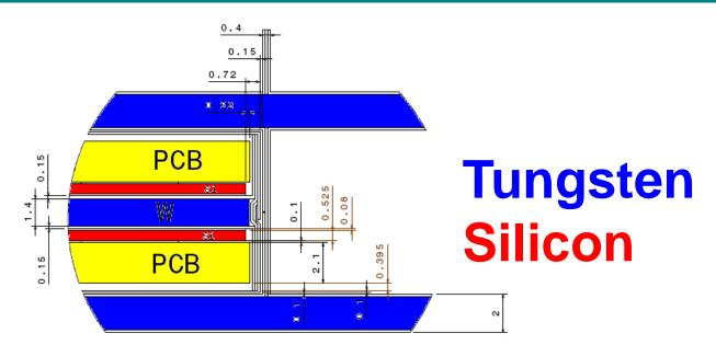
Odd and even layers have different material due to the PCBs
