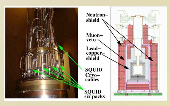
March 2004 operation stopped to install neutron veto, 66 channel SQUID readout to enable operation of 33 detector modules.
