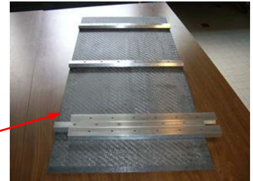
15mm thick plate with its rails; ready to be assembled with alveoli layers
