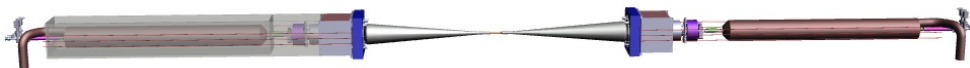
FIGURE 1.5-4. Interaction region of the ILD detector. The outer support structure of the magnets and forward calorimeters has been removed on the right side in this picture.
