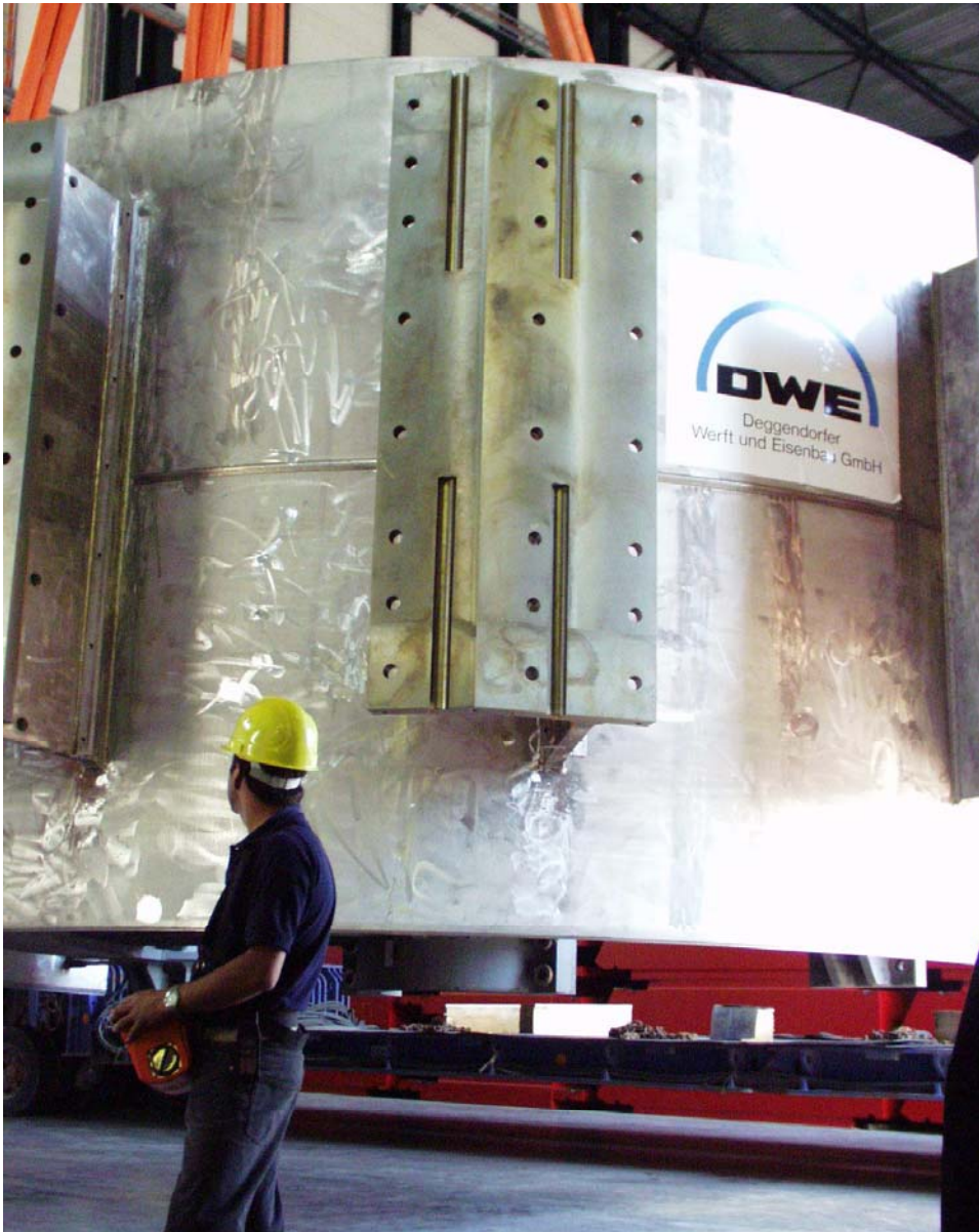
Vacuum tank with deep drilling for shear forces
