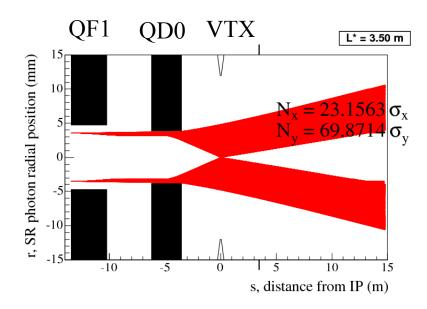
$\beta^*_{x,y}$  = 6.9, 0.07 mm  $\epsilon_{x,y}$  = 660, 20×10-9 m.rad  $E_{beam}$  = 1.5 TeV Constraining aperture is QD0 (3.8 mm) Fan remains < 10 mm at 15 m from IP Correction for dispersion  $\rightarrow$ 16  $\sigma_x$ , 70  $\sigma_y$
