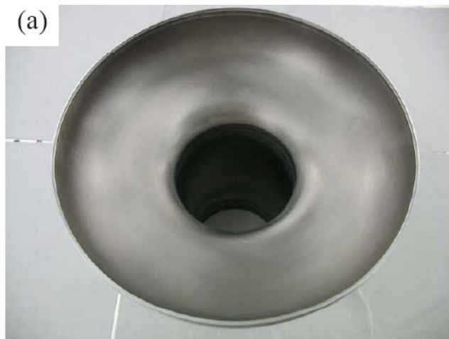
(a) Fine grain and (b) large grain half-cells after the iris weld.
