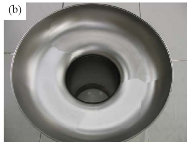
(a) Fine grain and (b) large grain half-cells after the iris weld.
