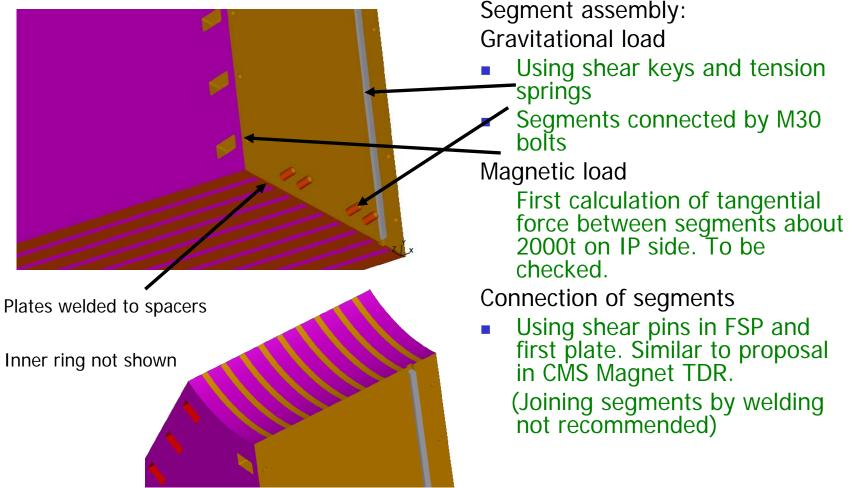
Connections of segments using plates and shear pins on first and last plate and FSP
