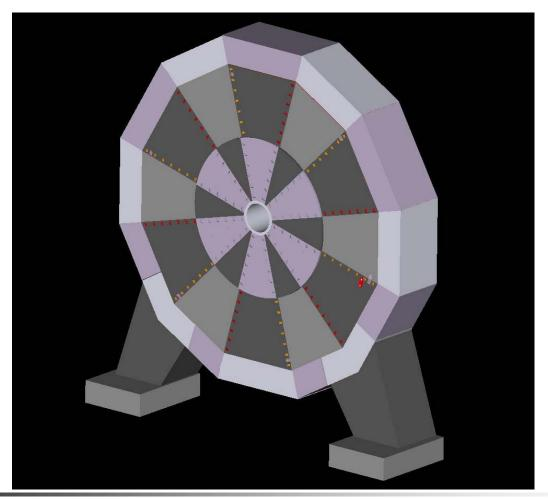
End-cap assembly inner ring, outer filling pieces and muon chambers
