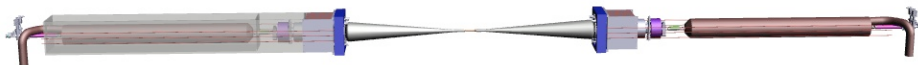
FIGURE 7.1-1. Interaction region of the ILD detector. The outer support structure of the magnets and forward calorimeters has been removed on the right side in this picture.
