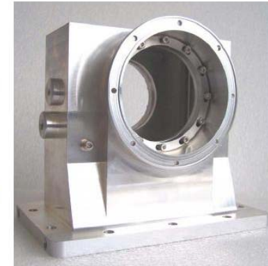
Al alloy: 1 single part - Prototypes: machined from single block - Mass production: casting + final machining
