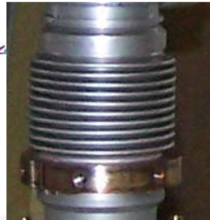
Copper + stainless steel + brass: 13 parts brazed and soldered
