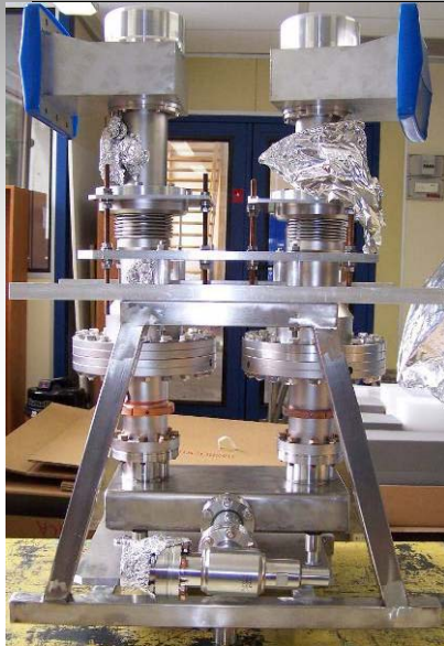
TTF-V coupler pair assembled for the RF tests
