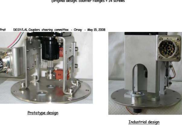
Design to minimize assembly time (original design: counter flanges + 14 screws)
