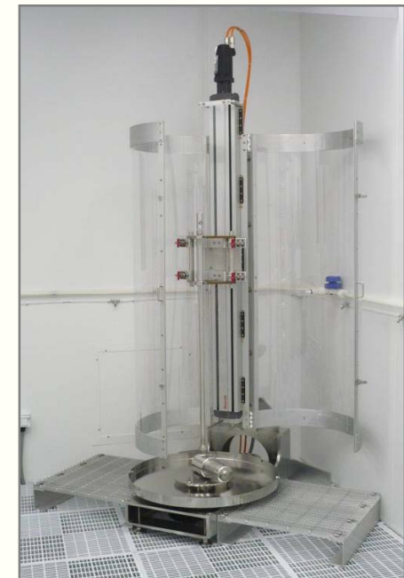
New High-pressure rinse system
