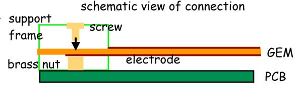
unmounted GEM module show the same problem once we establish HV connection (just unscrew-screw) HV connection was OK until we tighten screw of mounting bracket. -> the same problem again Our module may touch somewhere(dummy module?) in TPC????? and GEM might be displaced a little.
