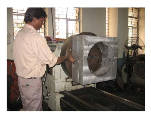
Left: The Shell being machined. Right: Machining of the Aluminium Fixture for holding the Shell.
