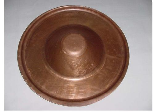
Second punch for forming the nose (on the left) and closer view of the End Wall formed in copper (right). A separate attachment for forming the End Radius (where the End Wall meets the Shell) has also been made.
