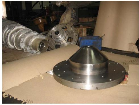
End Wall Die and one piece formed in copper (left) and first punch (on the right, in the foreground)
