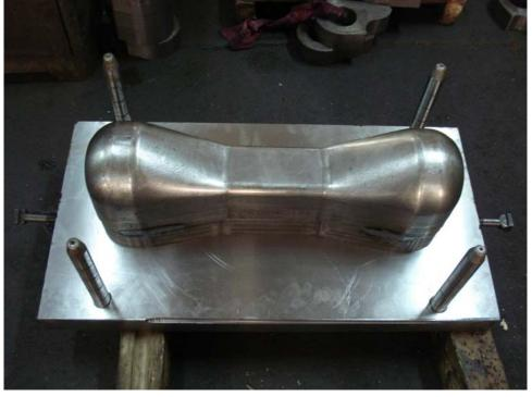
Die & Punch for forming the Half Spoke. The forming is actually done in two stages. In the first stage the central flat portion is formed (the die set for that is not shown here) followed by the full Half Spoke.
