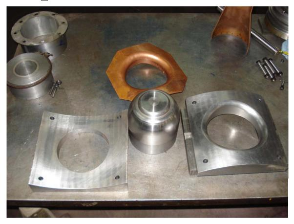
The Die & Punch for forming the Spoke to Shell Collar has been made. The trial copper piece formed has come out well. Measurements on the thickness at the EBW edge will be made shortly after it has been machined.
