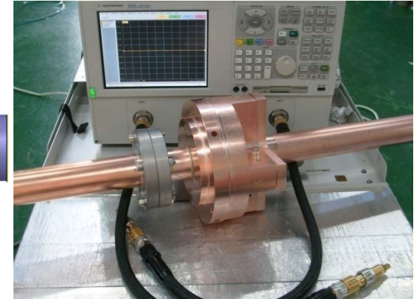
S-Band cavity BPM for ATF2 (KNU-LAPP-RHUL-KEK)
