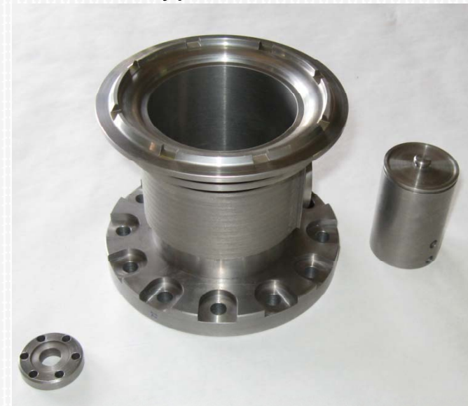
Prototype in Low RRR Nb
