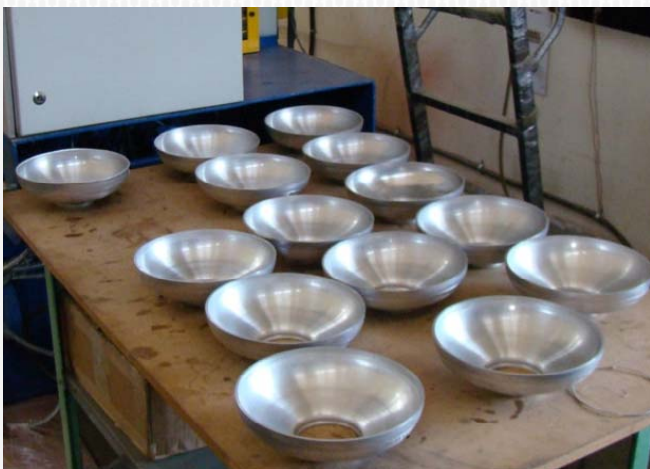
Forming of Al Half Cells
