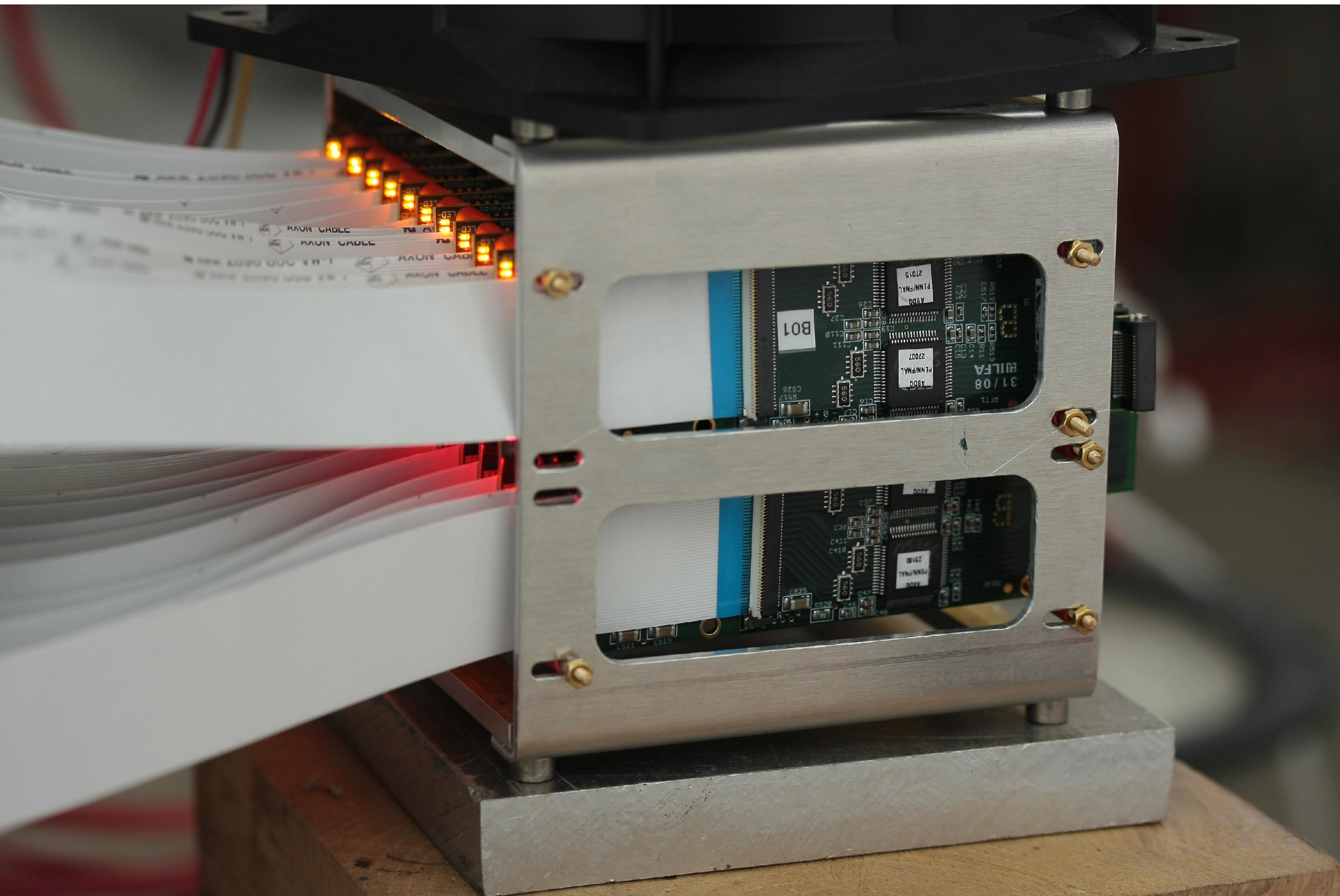
Barcelona board B09: cable displaced during assembly – no LV control available
