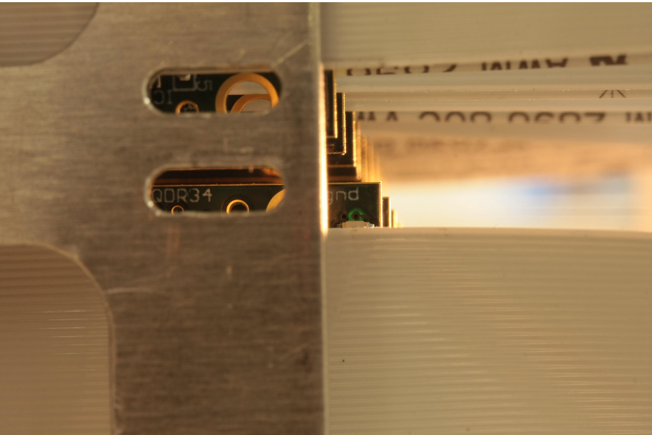
10 Barcelona boards connected to the GEM panel
