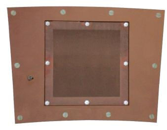
Module wit 2 Quadboards is finished, first cosmic tracks have been observed in test detector
