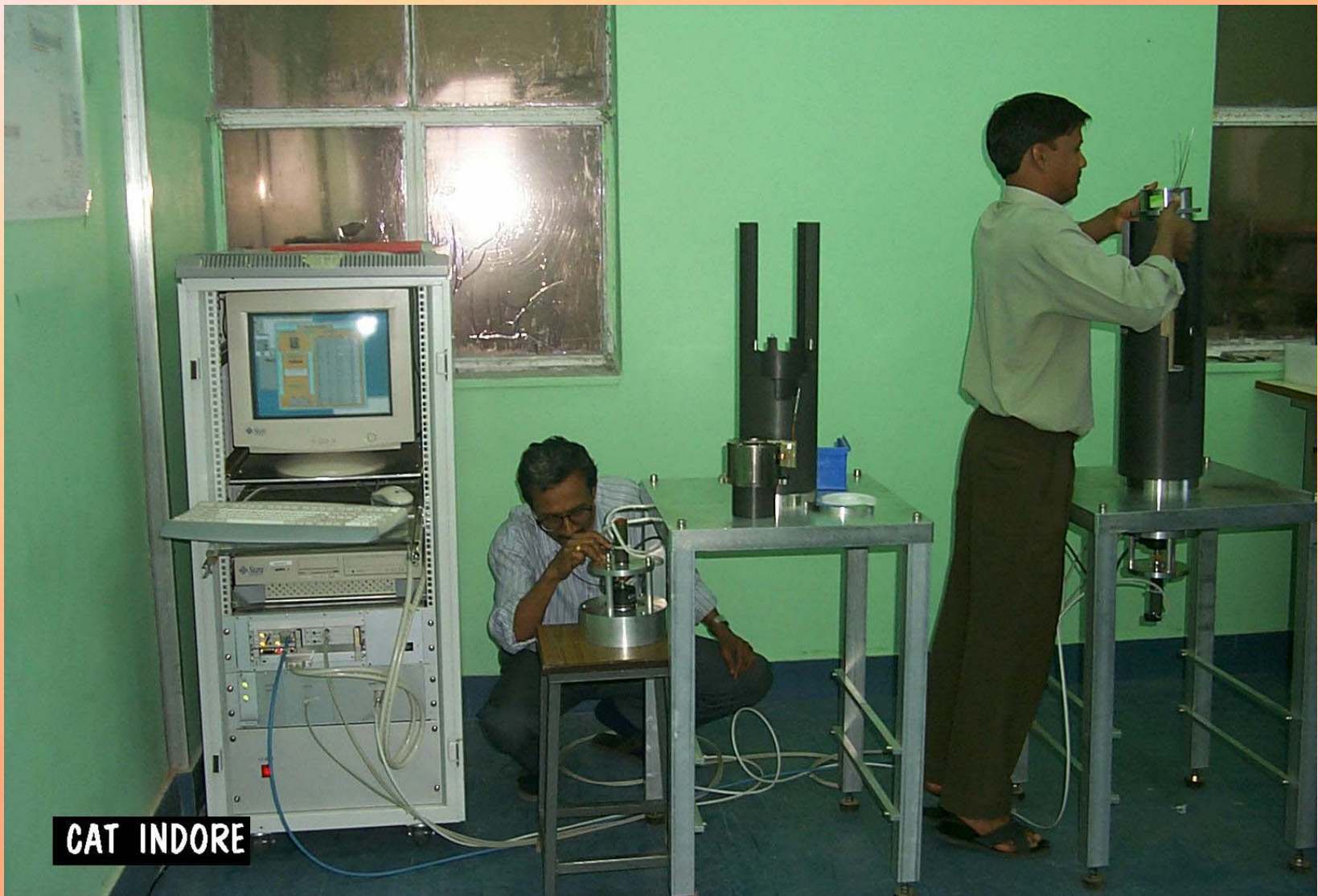
Magnetic measurement setup(WMM) for characterization of MCS magnets
