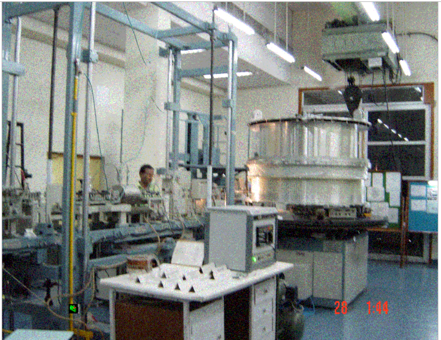
Coil Winding Set Up for K- 500 Superconducting Cyclotron Magnet Coil
