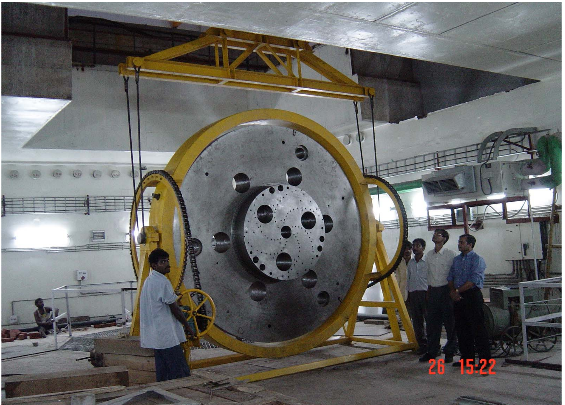
Top cap of magnet for superconducting cyclotron, Kolkata
