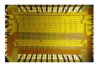
8 channels prototype produced
