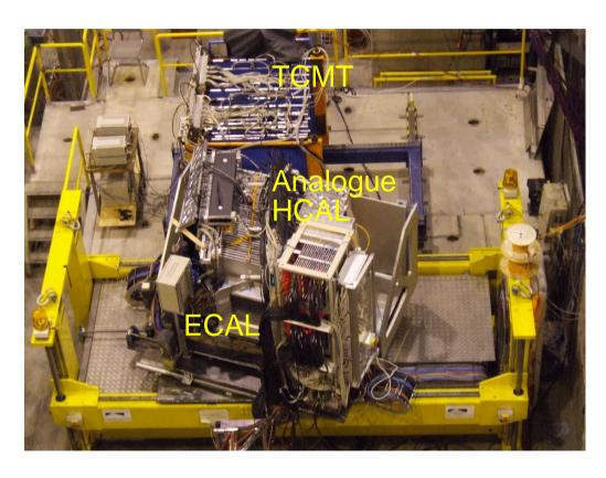
O(15000) calorimeter cells readout by Calice DAQ
