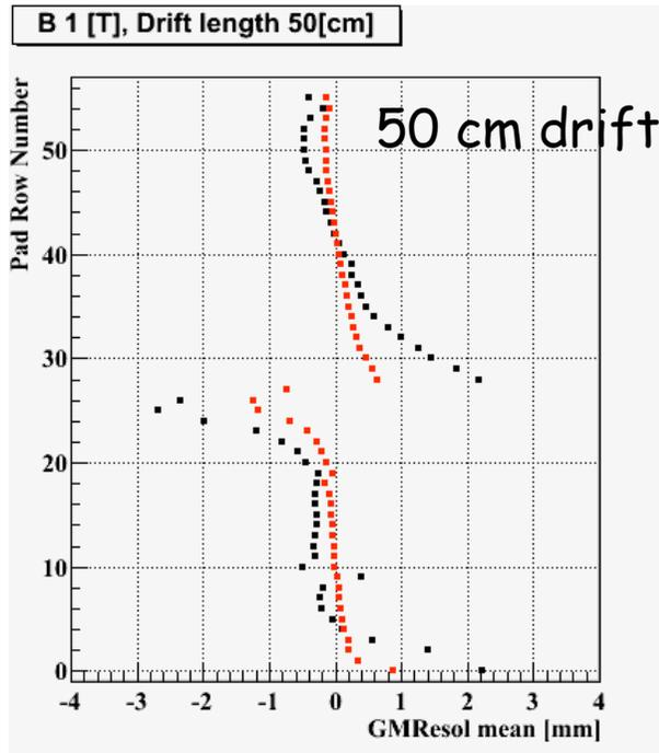
Metal posts facing drift volume produce local distortion.
