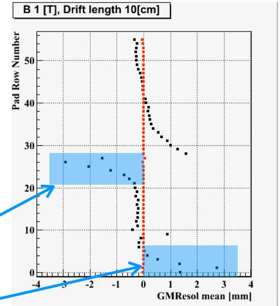
Poor resolution for module 1
