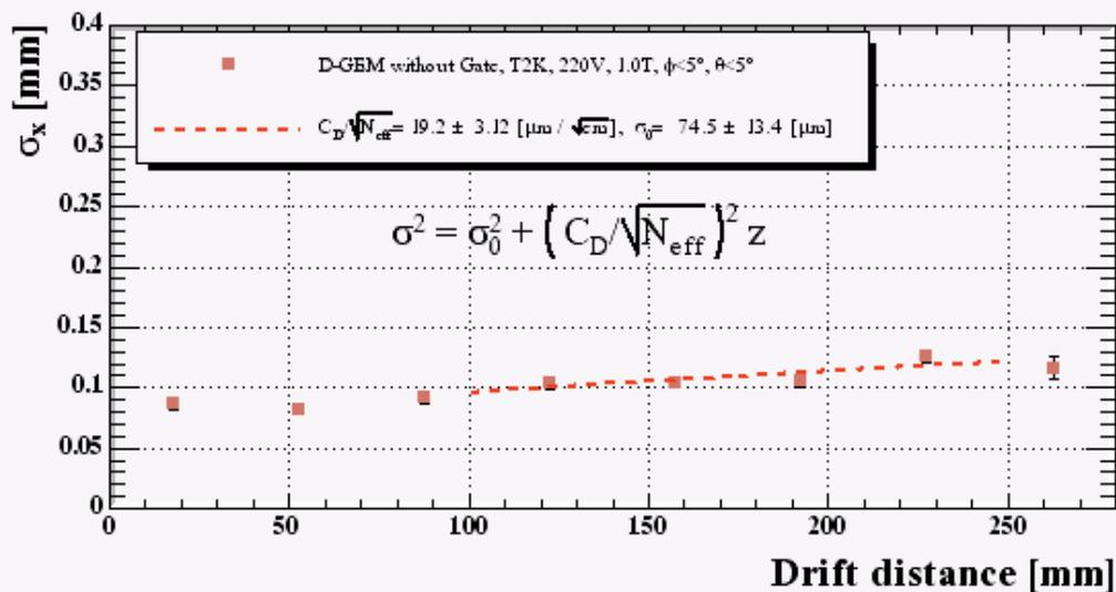
Result from small Prototype(MPTPC) with same condition except electronics
