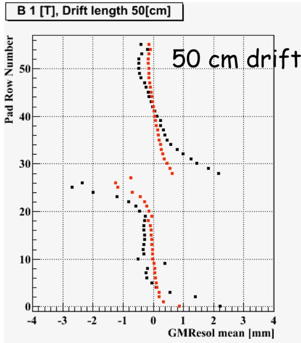
Data at 50 cm drift shows clear deviations even after correction
