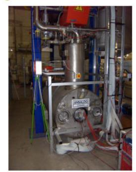
old ZEUS compensation magnet supraconducting solenoid reaches up to 5 T
