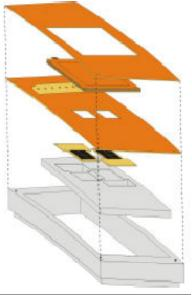
Triple-GEM module with readout by 8 Timepix chips: 16 cm2 active area, 0.5M channels
