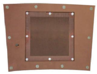
Gas amplification stage: 3 standard CERN GEMS (60/70/140) 1 mm spacing between GEMs
