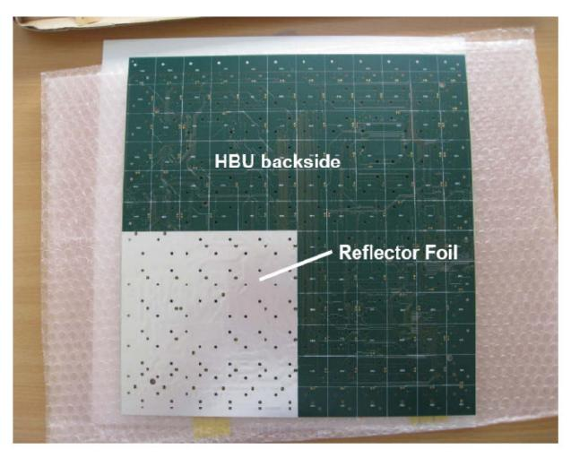
Cover back side with reflector foil in 4 pieces for better precision in alignment with holes
