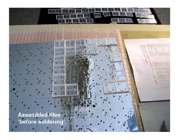
18 tiles connected and electronically checked All tiles available to equip full HBU
