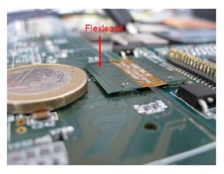
About 40 connection cycles up to now - still ok. Compensate HBU misalignments in distance.
