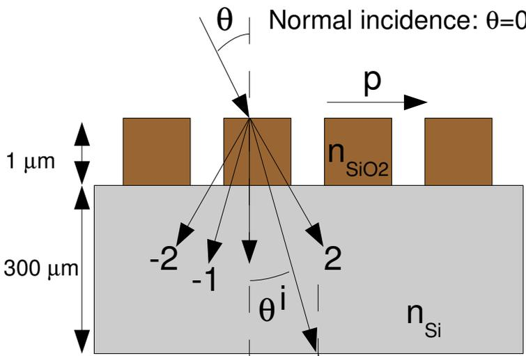
Propagation angle of diffraction order  $i$ :  $\theta_i$
