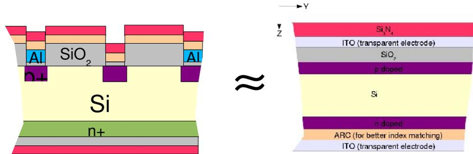
• **Simple simulation: multiple reflections**  $\Rightarrow$  interferences  $\Rightarrow$  Calculation of (T,R)
