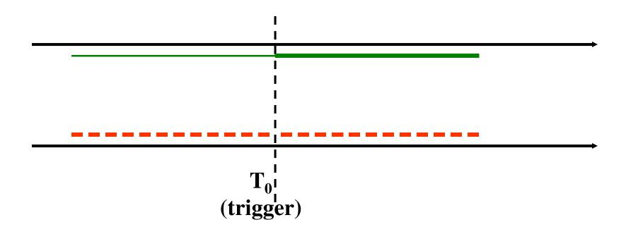
For M25 as a DUT, we may propose multiple readout after an <u>before</u> the trigger, in order to have the same sensitivity time. This is possible, because TNT-DAQ readout has no dead time!
