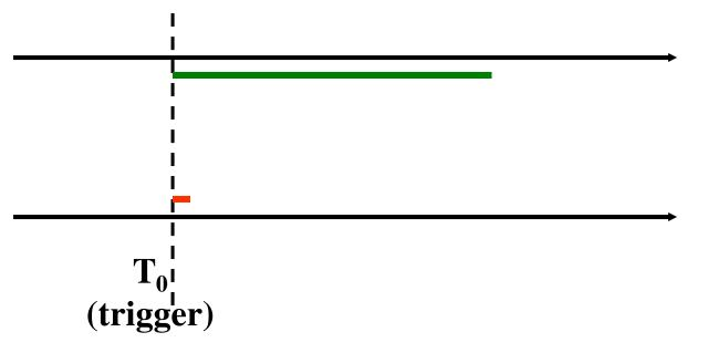
In addition, to avoid <u>multiple tracks</u>, no another trigger during 4 ms following T<sub>0</sub>.
