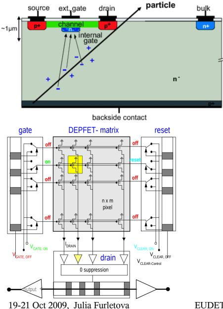
fully depleted sensitive volume, charge collection by drift require a -20 different voltages
