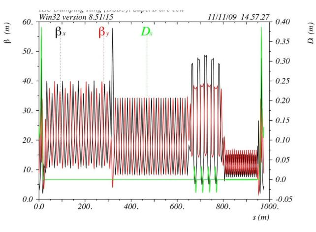
The wiggler straight is located downstream of the RF cavities in order to avoid damage by synchrotron radiation
