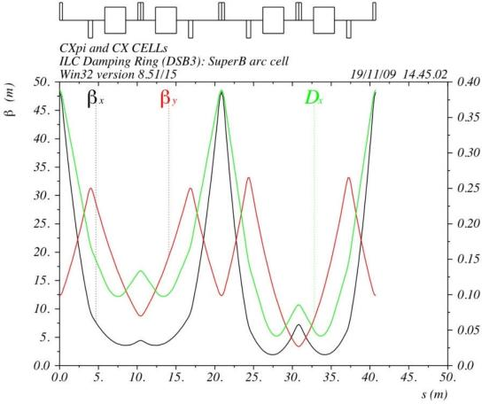
The arc lattice is based on the SuperB arc cells.
