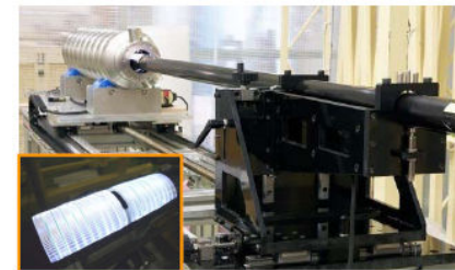
Strip line illuminator: LED+Light Guide Plate
