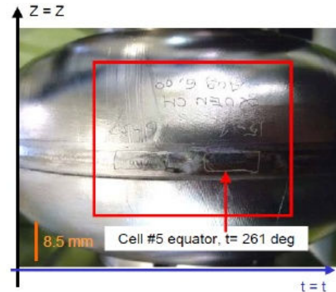
Limiting defect is weld repair – geometric flaw!
