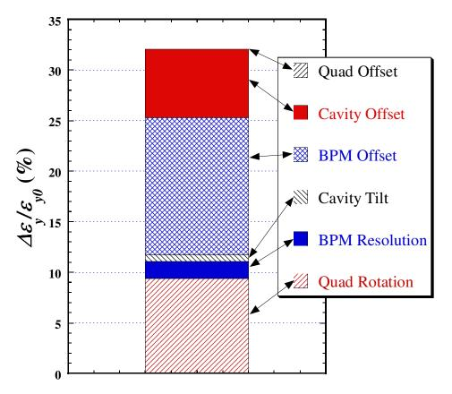
For 15 → 250 GeV ML, error set "equivalent to standard" The total and contribution of each error should be different if initial energy is 5 GeV.
