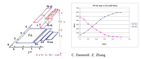
Potential under the output gate is pulled up by output node at 5 V
