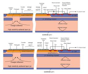
Figure: Upper: Surface Channel reset transistor; Lower: Buried Channel reset transistor. (K. Stefanov)
