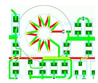
Less RFI, not sensitive to magnetic field – tested up to 4T
