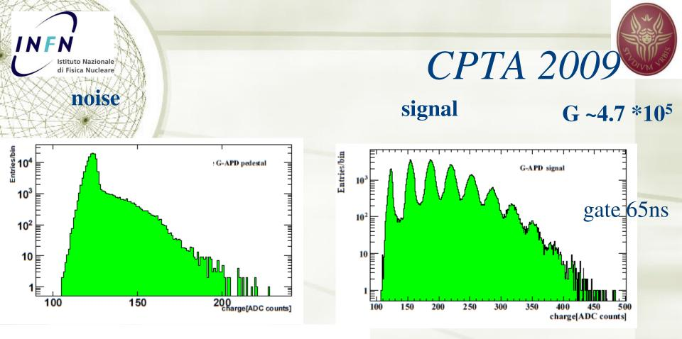
$N(x) = N \times \sum_{n} (\text{Gauss}(x, \mu_n, \sigma_n) \times \text{Poisson}(n, \lambda)) \text{const} \times e^{-\lambda} \sum_{n} (\lambda^n/n! \ 1/\sigma_n \exp\{-(x-\mu_n)^2/(2\sigma_n)^2\})$  **Real situation:** + Termogeneration  $\rightarrow \sim 30\%$  our timing + After-pulsing  $\rightarrow$  minor compared to Termogener. + Cross-talk  $\rightarrow$  much lower than Hamamatsu Simonetta Gentile, LCWS10, 26-30 March 2010, Beijing, China. 21 Istituto Nazionale di Fisica Nucleare
