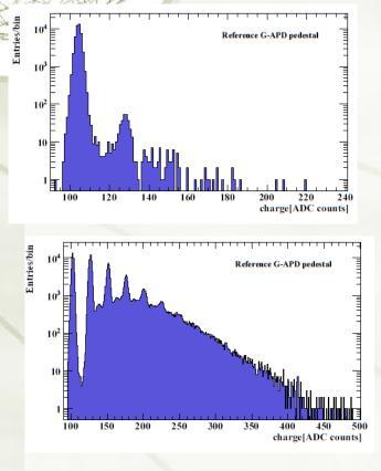
+Hamamatsu MPPC: S10362-11-025U  $G \sim 3.4 \ 10^5$ ✦ AfterPulse depending from gate lenght Gate = 65 ns Events/bin 10 10 100 150 200 250 300 charge [ADC counts]
